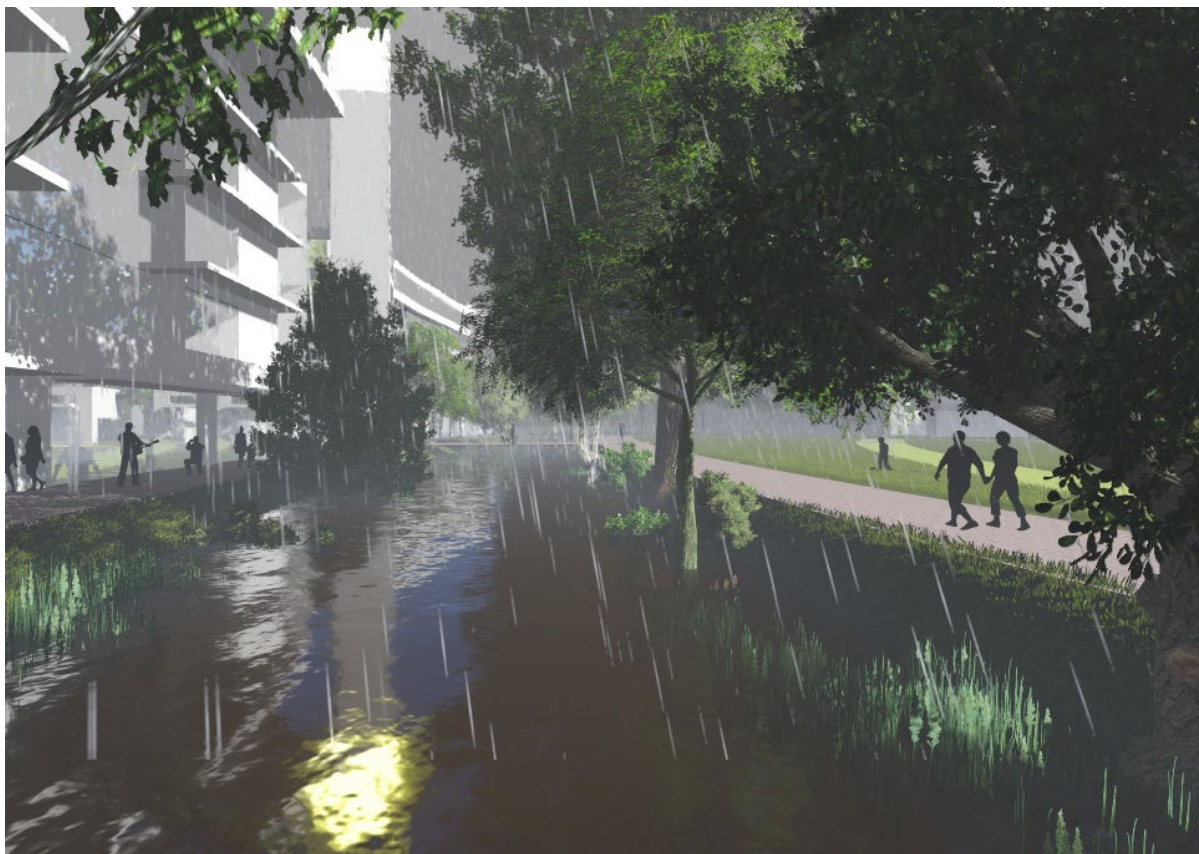
FIGURE 4 (RIGHT AND ABOVE): THE RUN BIOSWALE This engineered creek-bed will be a centerpiece of the Twin Aire Drive-In redevelopment. The bioswale will be lush with native trees and plantings, operating as a sponge during hydro-logical events (bottom).
